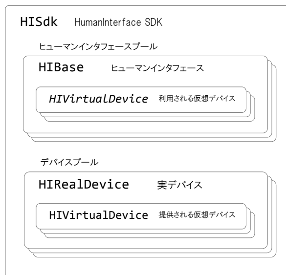
Fig. 10.2 HumanInterface module data structure
