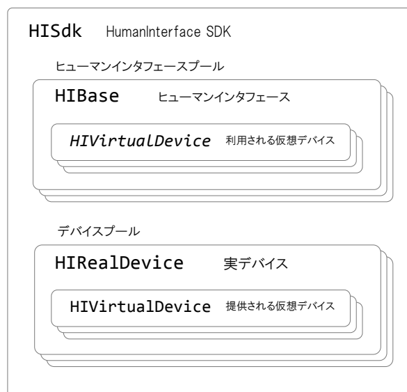
Fig. 10.2 HumanInterface module data structure
